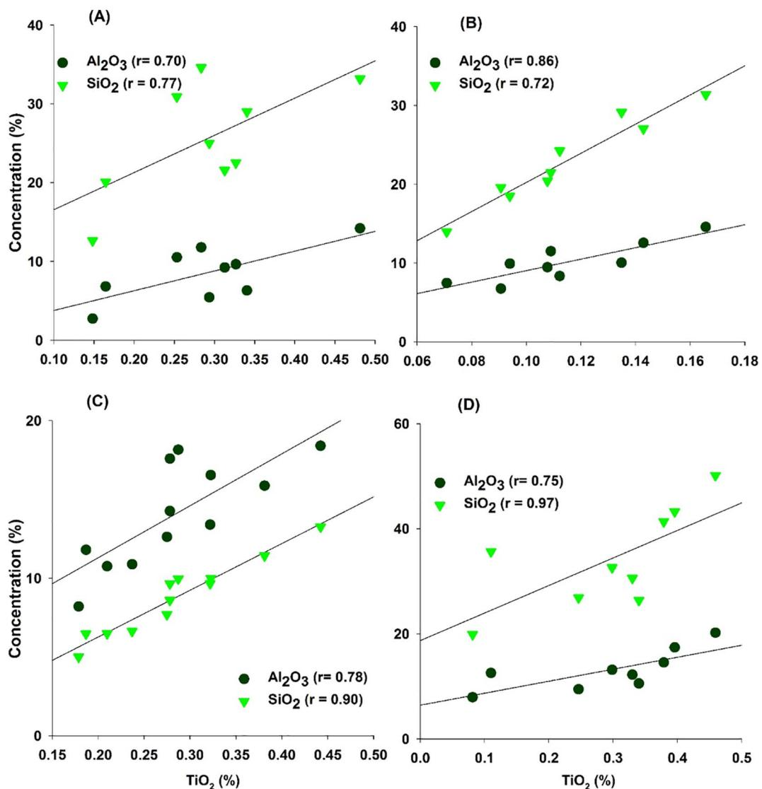
Fig. 5. Correlation between Al<sub>2</sub>O<sub>3</sub> vs. TiO<sub>2</sub> and SiO<sub>2</sub> vs. TiO<sub>2</sub> for samples from the (A) Padhrar coals, (B) Kotli coals, and (C) Block 3, (D) Block 5 of the Thar coalfield.
