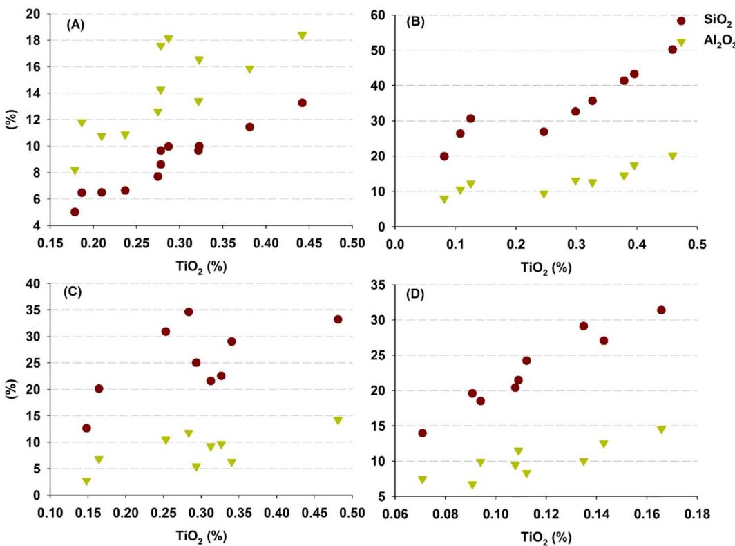
Fig. 4. Al<sub>2</sub>O<sub>3</sub> vs. TiO<sub>2</sub> and SiO<sub>2</sub> vs. TiO<sub>2</sub> for coal samples from the (A) Padhrar, (B) Kotli, and (C) Block 3, (D) Block 5 of the Thar coalfield.
