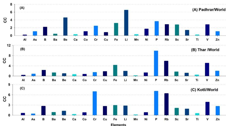
**Fig. 8.** Concentration coefficients of trace elements in the (A) Padhrar coals vs. world hard coals, (B) Thar coals vs. world hard coals, (C) Kotli coals vs. world hard coals. Data for trace elements in world hard coals are from Ketrus and Yudovich (2009).
