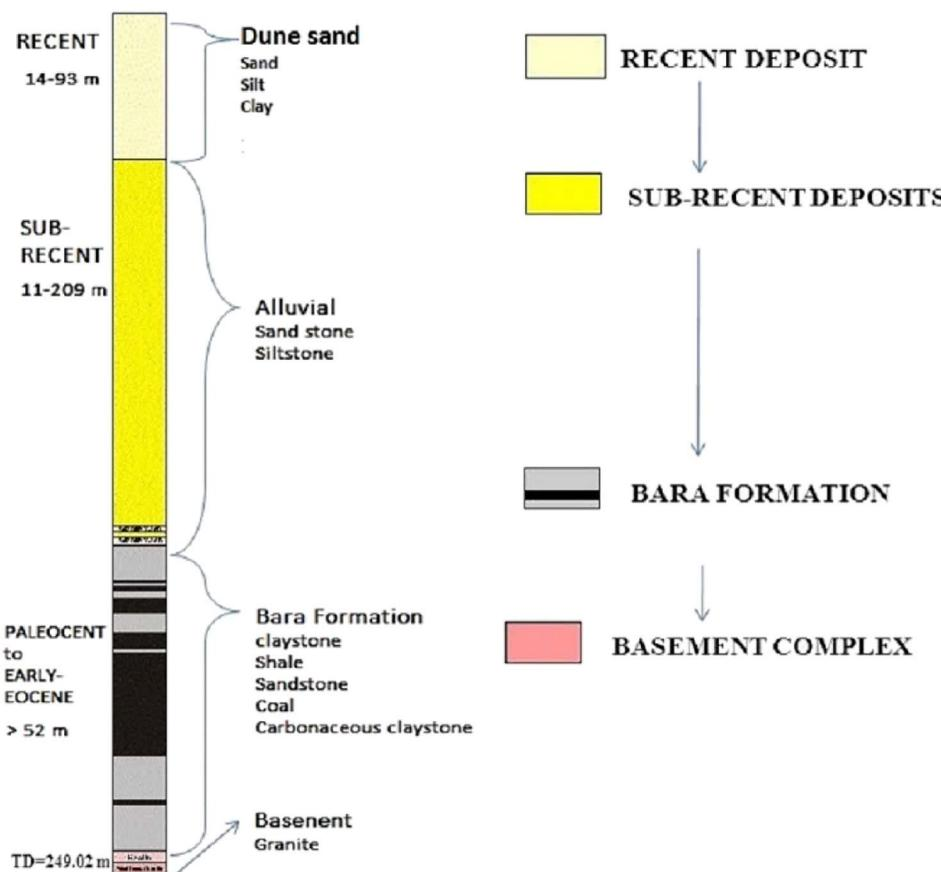
Fig. 2. Generalized stratigraphic column of the Thar coalfield.
