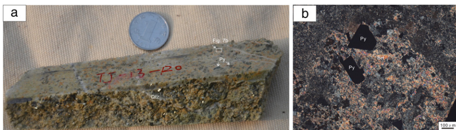
Fig. 7. (a) Photograph of silicification, sericitization and pyritization in sample TJ-13-120 from the Mashan ore section; (b) photomicrograph of the rock shown in (a). Abbreviations: Srt–sericite and others are as Fig. 4.
