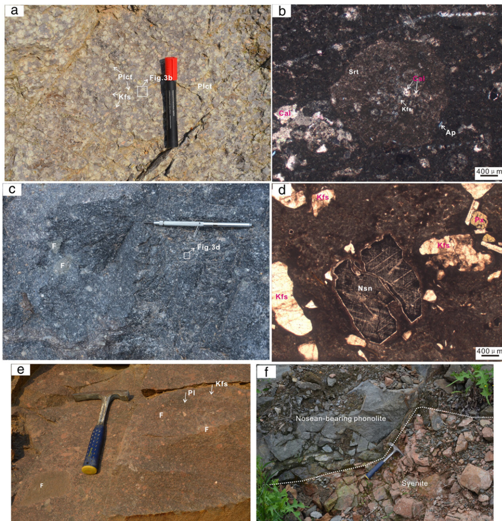
Fig. 3. Photographs and photomicrographs of the main rocks of the Niangniangshan Formation from the Tongjing Cu–Au deposit. (a) pseudo-leucite phenolite with porphyritic texture; (b) photomicrograph of the rock in (a), showing a leucite phenocryst completely replaced by sericite, K-feldspar and calcite, cross-polarized light; (c) nosean-bearing phonolitic brecciated tuff consisting of fragments of volcanic rock and crystal fragments set in a tuffaceous groundmass; (d) photomicrograph of the rock in (c), showing crystal fragments consisting of nosean, K-feldspar and pyroxene set in a tuffaceous groundmass, plane-polarized light; (e) trachytic volcanic breccia consisting of fragments of volcanic rocks and crystal fragments of K-feldspar and plagioclase set in a tuffaceous groundmass; (f) aegirine–augite syenite intruding nosean-bearing phonolite. Abbreviations: Plct–pseudo-leucite, Kfs–K-feldspar, Pl–plagioclase, Srt–sericite, Cal–calcite, Ap–apatite, F–fragment, Nsn–nosean, and Px–pyroxene.
