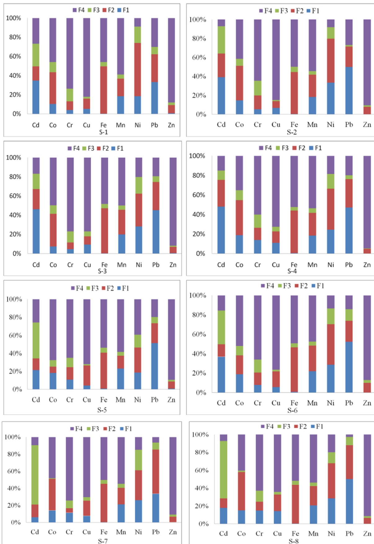
Fig. 2. The percentages of metal fractionations in sediments at different sites (S-1 to S-8).
