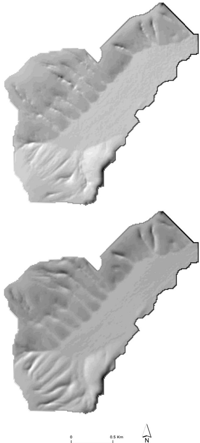
Fig. 12. Composite landform from an average of 100 simulations (top) and composite landform of maximum depths at 10,000 years using Waste Rock Dump parameters (bottom).
