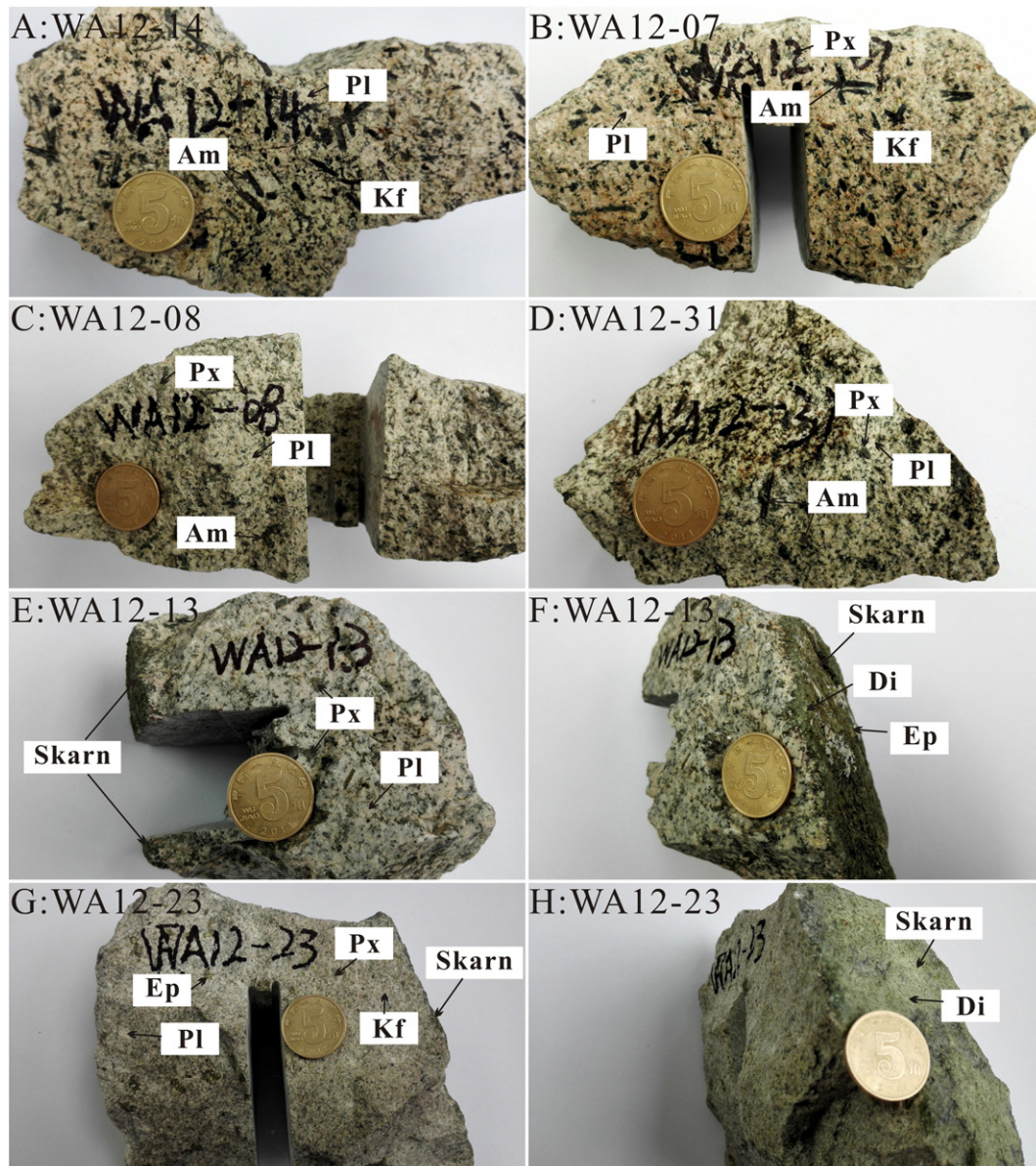
Fig. 2. Hand specimens of altered diorites and ores from the Han-Xing Fe skarn deposit. Abbreviations: Am-amphibole; Px-pyroxene; Di-diopside; Mgt-Magnetite; Kf-K-feldspar; Pl-plagioclase; Ep-epidote; Py-pyrite; Cal-calcite.
