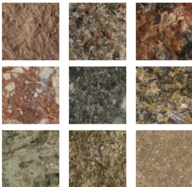
Fig. 2. Sample images from dataset. Each sample stands for one class. All images have size of 128 \times 128 \times 3 pixels and are between 1 and 2 cm across. From top to bottom, the first column – rhyolite, volcanic breccia, limestone; the second column – granite, andesite, oolitic limestone; the third column – red granite, peridotite, dolostone.
