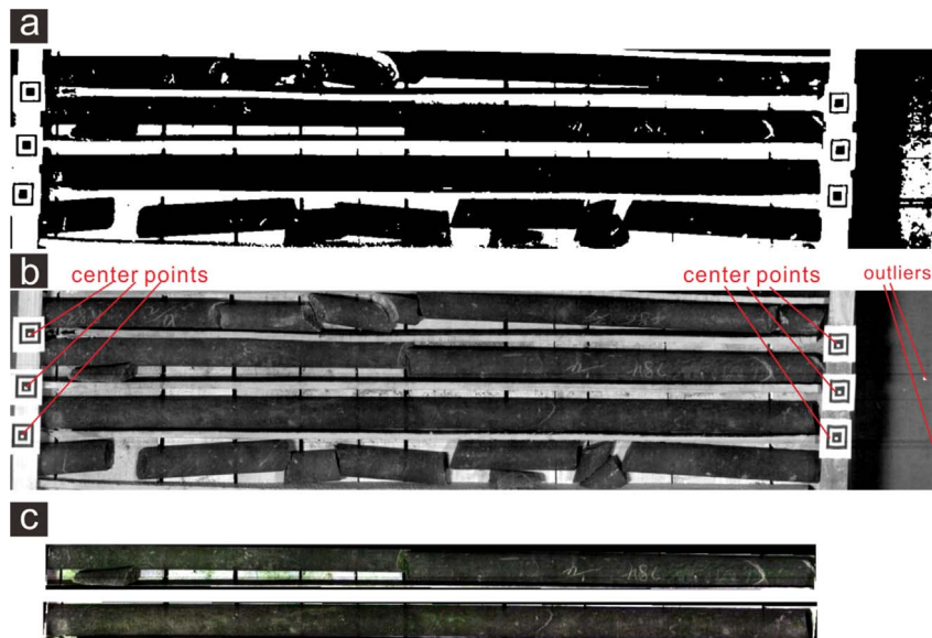
Fig. 14. Imaging of cores within a core box. (a) Monochrome image; (b) Marker identification image showing the center points identified by the program, including two false positives. (c) The resulting subset core image.
