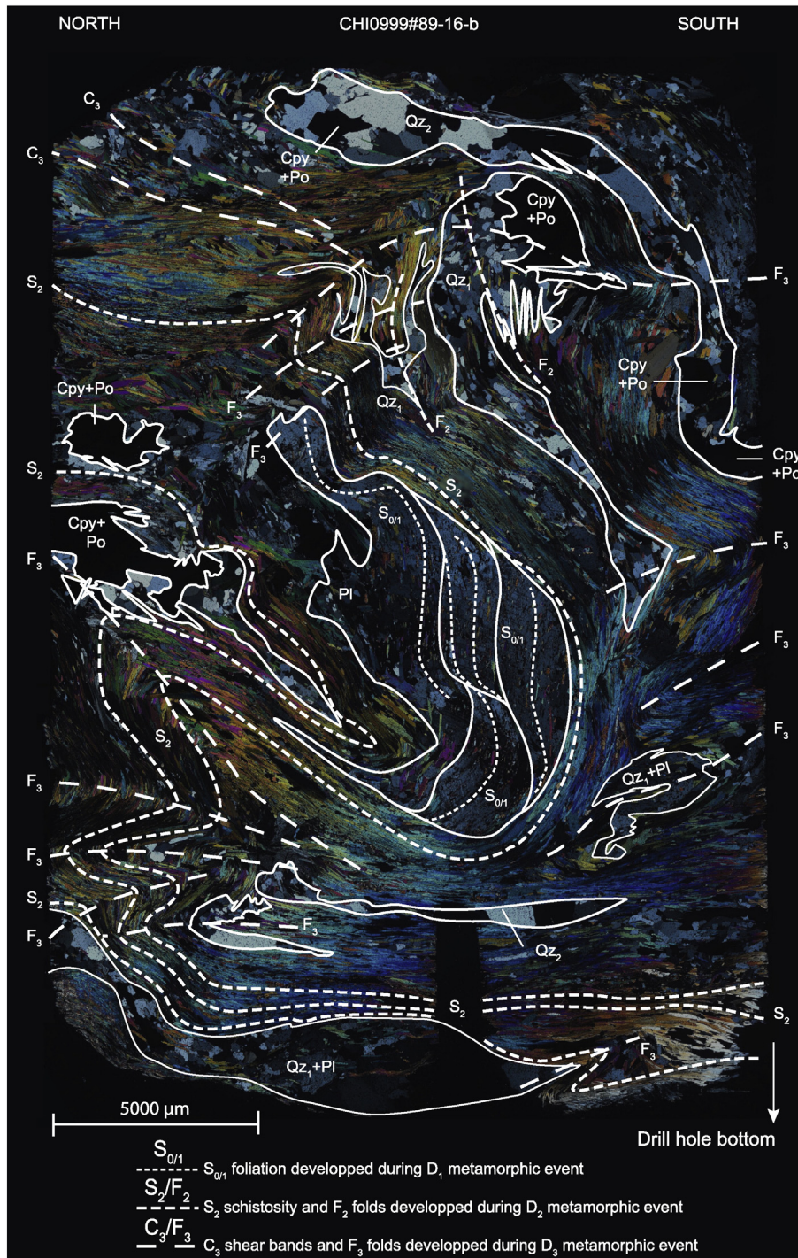
Fig. 6. Photograph of sample CHI0999#89-16-b under microscope (polarized and analyzed light) interpreted by adding the three metamorphic event microstructures. Abbreviations: Cpy = chalcopyrite; Pl = plagioclase; Po = pyrrhotite; Qz 1 = first generation of quartz; Qz 2 = second generation of quartz.
