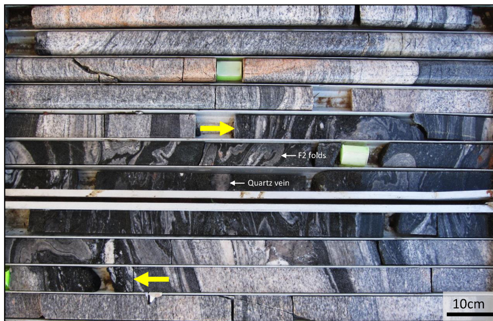
Fig. 7. Photograph of drill core from Omitiomire to illustrate the heterogeneity of strain in the deposit. In this example, high strains are confined to a 6 m wide zone (between arrows) of transposed biotite–epidote schists. Note the F2 folds and quartz veins associated with the high strain zone.
