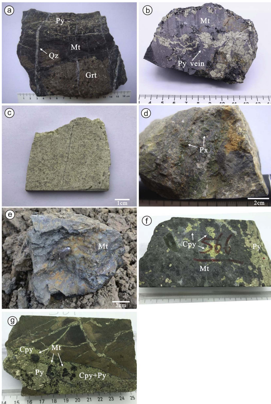
Fig. 4. Photographs of hand-specimens from the Beiya deposit showing mineralogy and textures of the five samples used in this study. (a) Typical skarn mineralization of the Beiya deposit. The early garnet was replaced by late magnetite, and the magnetite was then cut by the pyrite veinlets; (b) Magnetite ore cut by pyrite veins; (c) The ore-related quartz syenite porphyry collected from the open pit (M1); (d) Skarn with green pyroxene from the early retrograde alteration stage (M2); (e) Fe-oxide ore from the open pit dominated by massive magnetite with no sulfide (M3); (f) Massive magnetite ore coexisting with minor pyrite and chalcopyrite (M4); (g) Sulfide-dominated vein hosted within altered country rock, with minor magnetite coexisting with sulfides (M5). Abbreviations: Cpy-chalcopyrite, Grt-garnet, Mt-magnetite, Px-pyroxene, Py-pyrite, Qz-quartz.
