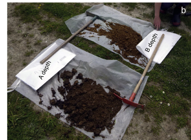
Fig. 2. The sampling methodology. a. Design of soil collection pattern at each field duplicate locality. Duplicates were collected at c. 1 in 20 randomly selected sites. b. Soil samples from the five auger holes were amalgamated in the field.
