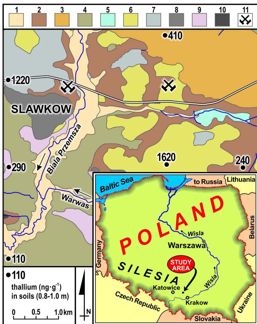
Fig. 1. Sampling points. Lithological background: (after Kurek et al., 1994) 1. flood plain sands, gravel and silts, 2. slope-wash sands and loams, 3. loesses, 4. glaciofluvial sands and gravel, 5. Triassic clays-tones and limestones, 6. Middle Triassic dolomites, limestones and marls, 7. ore-bearing dolomites, 8. Lower Triassic dolomites and marls, 9. Permian claystones, siltstones and conglomerates, 10. dumps, 11. abandoned Zn-Pb ore mines.
