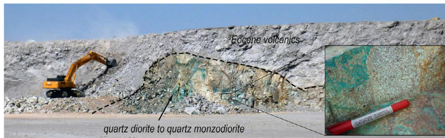
Fig. 5. The Chah-Firouzeh porphyry quartz diorite to quartz monzodiorite intruded Eocene volcanic rocks. Mineralization occurs as veinlet and stockwork system. The inset square show secondary mineralization as malachite that replaced in the fractures, as well as plagioclase phenocrysts in the Chah-Firouzeh porphyry.
